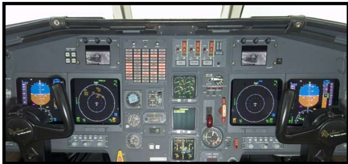
Figure1: AVDU-1010 in pilot and co-pilot positions on Falcon jet for EVS application
